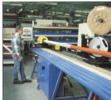
Automatic mandrel made hose with or without wire or nylon rod reinforcements in single or multiple fabric coatings.
