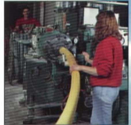
Extruding hose with multiple reinforcements of custom strands or fabrics.
