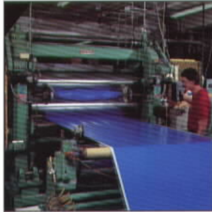
Calendering. We compound, mix and calender silicone and other exotic compounds to a wide array of reinforcing fabrics; single or double coatings, a range of durometers, precise thickness and widths.
