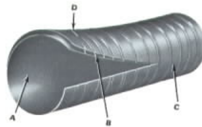
A. Neoprene/Fiberglass Inner Liner Ply B. Helical Coiled Spring Wire C. Neoprene/Fiberglass Cover Ply D. Double Fiberglass Cord
