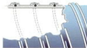
A. Silicone/Fiberglass Inner Liner Ply B. Helical Coiled Spring Wire C. Silicone/Fiberglass Cover Ply D. Double Fiberglass Cord
